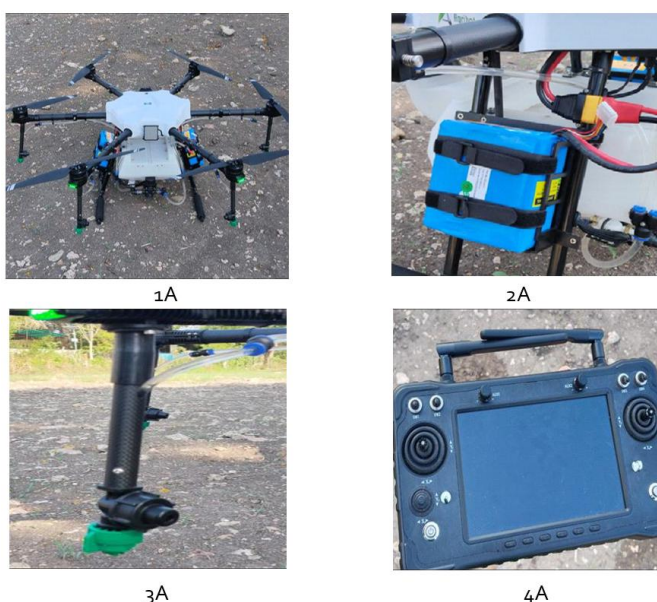
Fig. 1. 1A-Six-rotor agricultural spraying drone 2A- Battery set (Power source) 3A- Agricultural spraying nozzle 4A- Drone control unit (Remote controller) (Gadhe et al., 2025)
