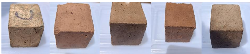
Fig. 11. Mortar cubes of Cement, LC 3 50% C 1 , LC 3 25% C 1 , LC 3 50% C 2 , LC 3 25% C 2
