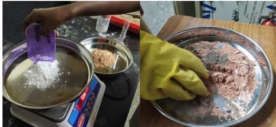
Fig. 8. Weighing and mix preparation for flow table test
