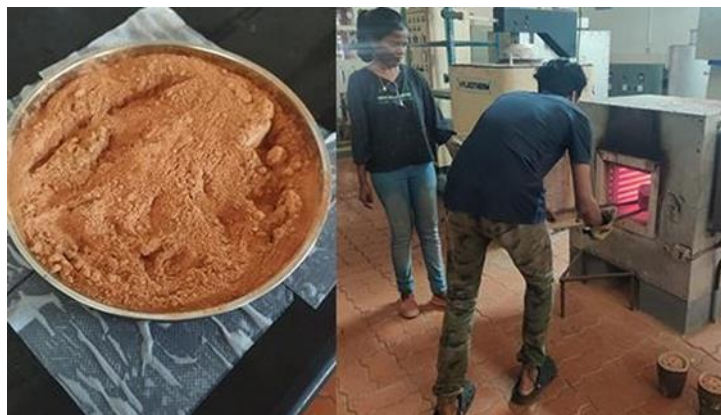
Fig. 5. Calcined clay and calcination of clays using muffle furnace
