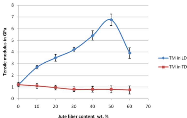
**Fig. 3.** Effect of jute fiber content on TM of JS/UPE composite in longitudinal and transverse direction
