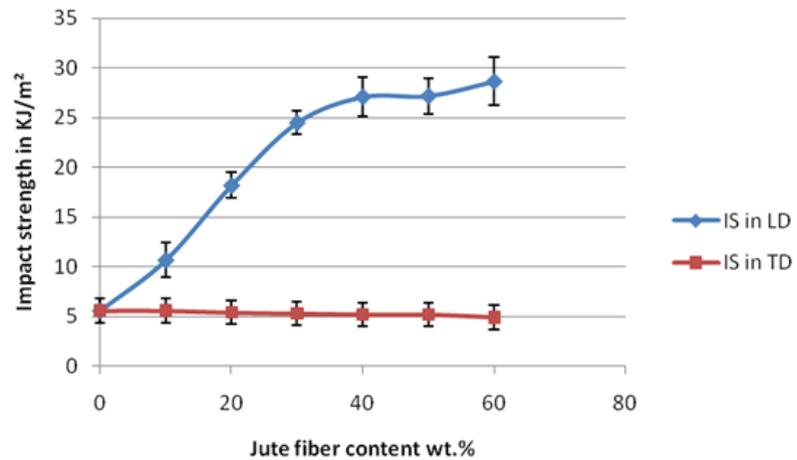
Fig. 6. Effect of jute content on IS of JS/UPE composite in longitudinal and transverse direction
