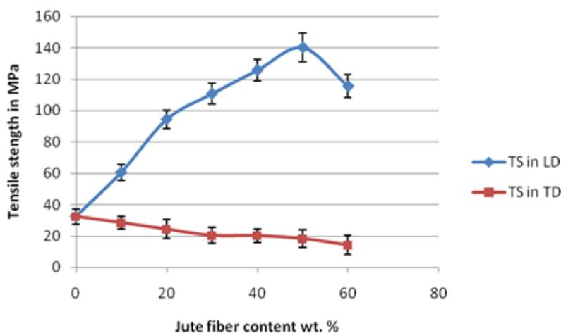
**Fig. 2.** Effect of jute content on TS of JS/UPE composite in longitudinal and transverse direction
