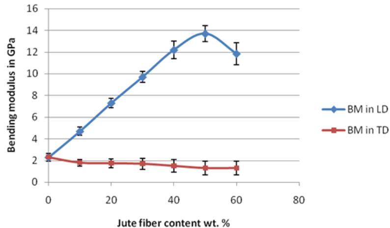
Fig. 5. Effect of jute content on BM of JS/UPE composite in longitudinal and transverse direction
