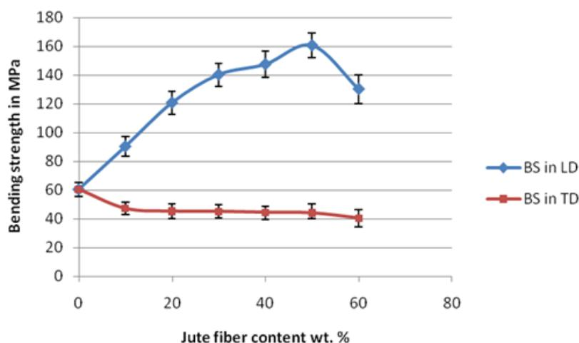
**Fig. 4.** Effect of jute content on BS of JS/UPE composite in longitudinal and transverse direction
