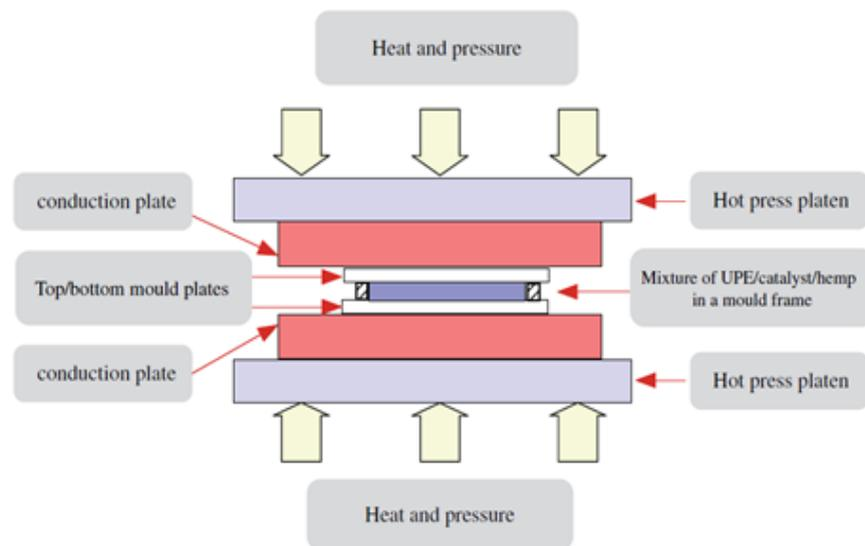
Fig. 1. Schematic diagram of the composite consolidation
